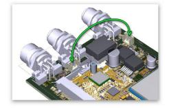
it is imperative that they have insulation between the CAN and the process side in accordance with EN50155!
