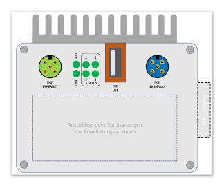
A 4-pole, D-coded M12 connector is used for the **Ethernet connection**, to which commercially available cables from Phoenix Contact, Metz Connect and other manufacturers can be connected.
