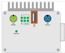
While the two 9-pin MVB connections can be found on the side of the fieldbus connections on the device, only one status display of the MVB module is additionally present opposite. On the MVB connections, pins 1 to 5 are connected between [X9] and [X10]. Pins 6 to 9 offer an option for standard-compliant termination of an EMD bus as standard.
